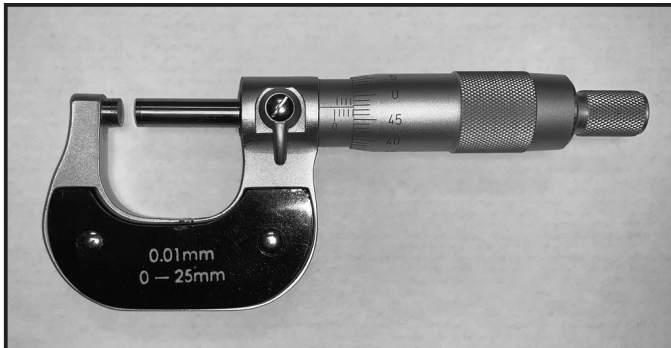
Micrometer (up to 25mm)
