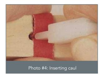
5. Position both pieces of cloth in the mortise, estimating 5mm depth. Holding the cloth against the top of the key, insert a bushing caul. Immediately remove the caul to check for proper cloth depth. Adjust as necessary, and then reinsert the caul (photo #4).
