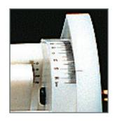
The rake angle is set by loosening the Locking Knob, pulling on the Spring Pin, and lining up the edge of the Rake Bar to the proper mark on the Rake Angle Gauge. The pin is set at 90° to make squaring up the rake for grands fast and easy. Rotate rake until it pops in place.
