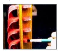
6. Size the bushings by wetting with alcohol and inserting a #7 bridge pin into each. Most damper wires measure .073", and #7 (.086") bridge pins size the bushings to a comfortably free fit. If you prefer a tighter fit, use #6 (.076") bridge pins. Place in a warm spot to dry for several hours. When the bushings are thoroughly dry, they will have uniform, firm holes free of fuzz that will control the damper wires with negligible friction.
