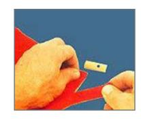
Once the correct width is determined, insert a piece into the hole, pull half of the strip through, and test the fit of the pin. It should be too tight to allow insertion by hand, but not so tight that the wood part is in danger of splitting. Select cloth thickness as needed. Once correct width and thickness are determined, use the end of the strip with the 1/2" cuts as a gauge for making starter cuts for any additional strips needed.
