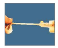
10. Cut the protruding pin flush with the wood.
