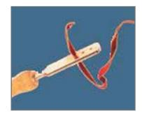
5. Activate the glue coating by wiping the outer surface of the cloth with a wet sponge. Then insert the cloth through the action part and pull through almost to the end of the cloth. Orient the seam of the cloth according to the Renner specification [Diagram 1 on last page of this manual]. If you are rebushing a number of parts, string them tight together on the same piece of cloth.
