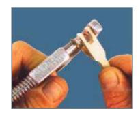
3. Clean out the bushing holes using the proper sized drill in a pin vise. For most parts, this will be a #39 drill (.0995"). You want to remove only cloth and glue residue, and not damage the wood. Best results are had by first turning the drill counter clockwise until it is through both flange ears, then forward a turn or two. This maintains the original alignment of the two holes.
